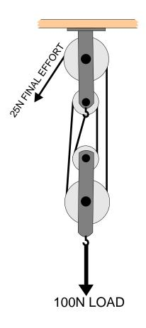
The pulley system opposite has 1:4 ratio (effort : load). An effort of 25N can lift a load of 100N.
