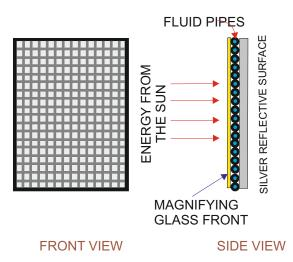
**4.** A modern solar panel, for heating domestic water is shown opposite. Explain how it works. **6 marks**
