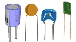
Capacitors are components that are used to store an electrical charge. They are often used in timer circuits. A capacitor may be used with a resistor to produce a timer. Timers are found in a large range of electronic devices
