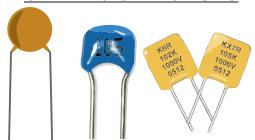
Non-electrolytic capacitors usually have a low capacitance compared to electrolytic capacitors.
