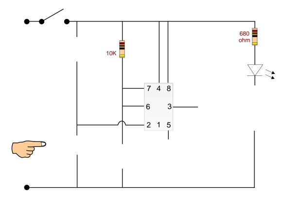
5. Describe how the monostable circuit shown above works. Include an explanation of the functions of the major components
