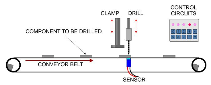
The timer circuit is found inside the control circuit box. The incomplete circuit diagram is found below. Add the following components to complete the timer circuit:
