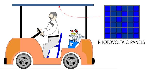
This is a solar powered golf cart and it can be used in sunny climates to carry golfers from one hole to the next. When it is standing still the solar panels charge up the batteries and it is the batteries that power the electric motors, directly. As the vehicle is not in continuous use the batteries have time to charge up before they are needed. This is ideal for my Dad as he plays golf and does not like walking.
