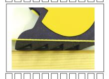
The rubber grip at the bottom of the casing looks good, but when tested it tended to slip. This was due to the tape measure being lightweight.
