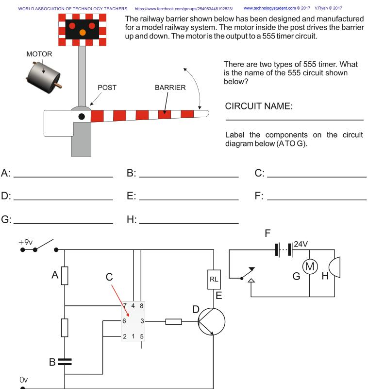
The relay is causing major problems because an important component is missing. Name the component and draw its symbol in the correct position on the circuit diagram above.
