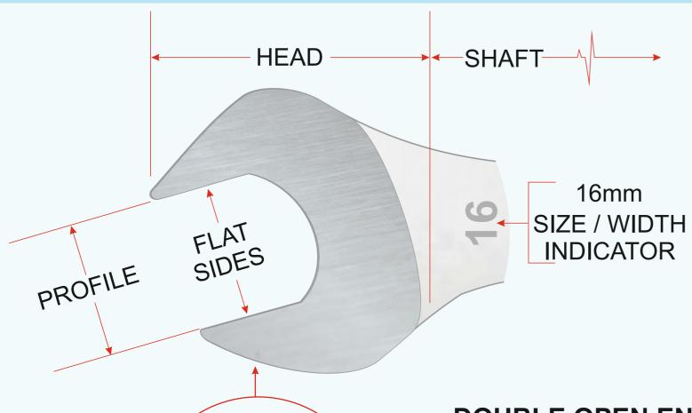
An open ended spanner, sometimes called a wrench, has a head with an 'open profile', normally at each end. Each of the profiles are different sizes and have flat, parallel sides. The head is normally angled at 15 degrees, which makes the rotation of the spanner easier. The spanner shown here is a double open ended spanner. Single open ended spanners are also available.
