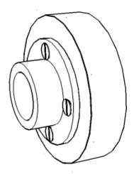
2. The sketch opposite, shows the blank being turned for the first time, in order to produce an accurate cylinder.
