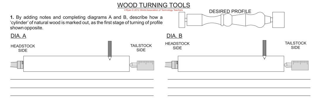
2. The profile (shape) of a turned piece of wood has been achieved using a range of lathe tools. Add a sketch of each of the tools you think were used to produce the various shapes. One of the tools has been drawn and named for you.
