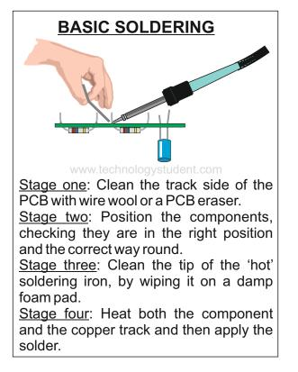
1. Describe soldering components to a PCB, in four simple stages.
