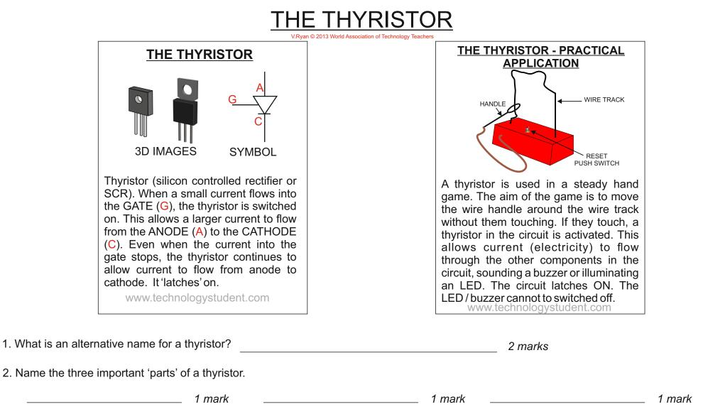
3. What is the sequence of events that leads to the thyristor switching on / latching on? 3 marks
