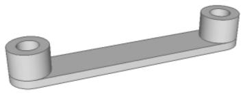
It has been decided that the plastic being used for the coupling wears out too quickly. Aluminium is to be used.
