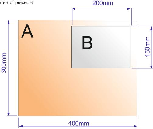
First, calculate the entire area of 'A', without the smaller piece being removed, by treating it as a rectangle 400mm x 300mm.
