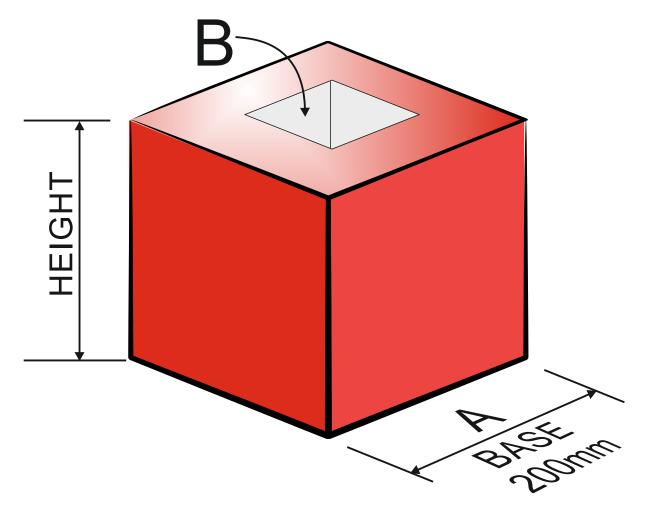
A solid cube of aluminium (A) has 200mm sides. However, a smaller area in the form of a cube with 100mm length sides, has been machined from the top surface (B). What is the volume of the finished 3D shape?
