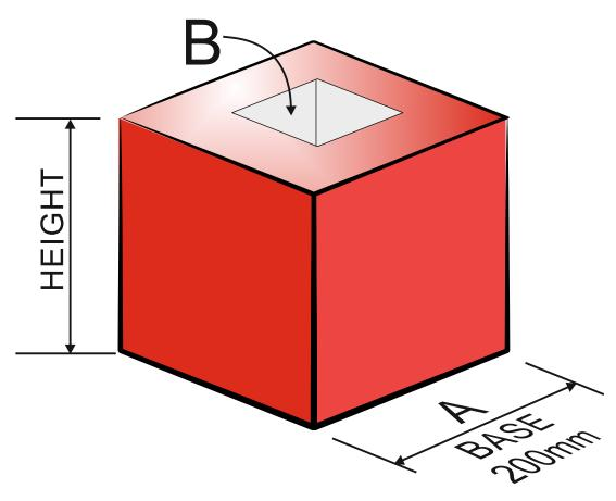
A solid cube of aluminium (A) has 200mm sides. However, a smaller area in the form of a cube with 100mm length sides, has been machined from the top surface (B). What is the volume of the finished 3D shape? Explain your working out.
