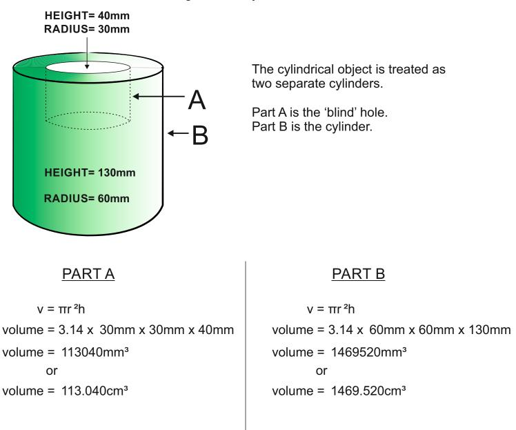
Then subtract the volume of part A from the volume of part B, to find the overall volume of the engineered object.
