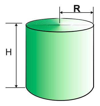
In order to calculate the volume of a cylinder, the height and radius of the circular top /bottom must be known. The following formula is used to calculate the volume.
