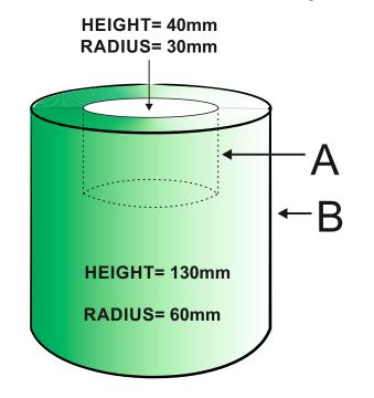
The cylindrical object is treated as two separate cylinders.
