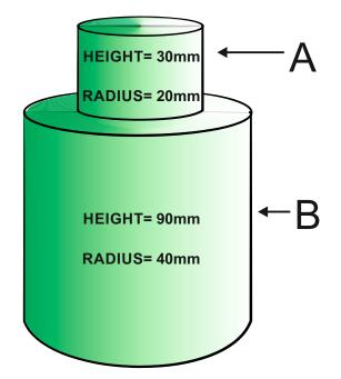
In order to calculate the entire volume of the engineered solid, it is treated as two separate parts. Part A is the smaller cylinder and part B is the larger cylinder.
