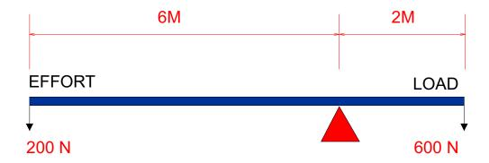
Clockwise moment = 600 x 2 Nm Anti-clockwise moment =  $200 \times 6 \text{ Nm}$ In a state of equilibrium, clockwise moments = anti-clockwise moments  $600 \times 2 \text{ Nm} = 200 \times 6 \text{ Nm}$ 1200 = 1200
