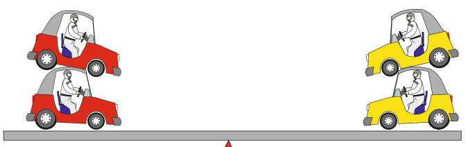
A state of equilibrium is also seen below. Each of the cars weighs the same (1 Tonne). Despite the fact that there is only one car on the left-hand side, the moments balance because, the car on the left-hand side, is twice the distance from the fulcrum, compared to the cars on the right-hand side. (see the calculation below).
