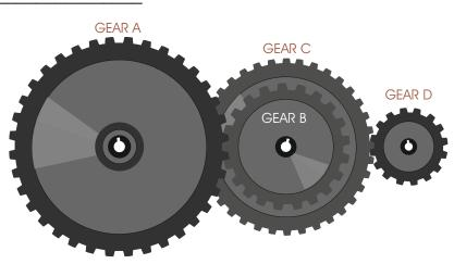
Gear A rotates in a clockwise direction at 30 revs/min. What is the output in revs/min at D and what is the direction of rotation?
