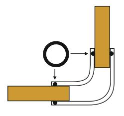
3b. The pipe connector, seen opposite, has 'O' rings to prevent leaks. Explain why an hydromorphic polymer is the best material to use in this situation. *4 marks*
