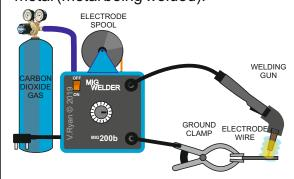
2. What is the purpose of carbon dioxide, during MIG welding?
