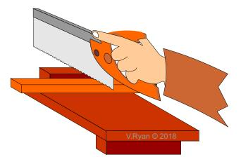
5. The diagram opposite shows a piece of wood, a bench hook and tenon saw. Describe the sawing technique.
