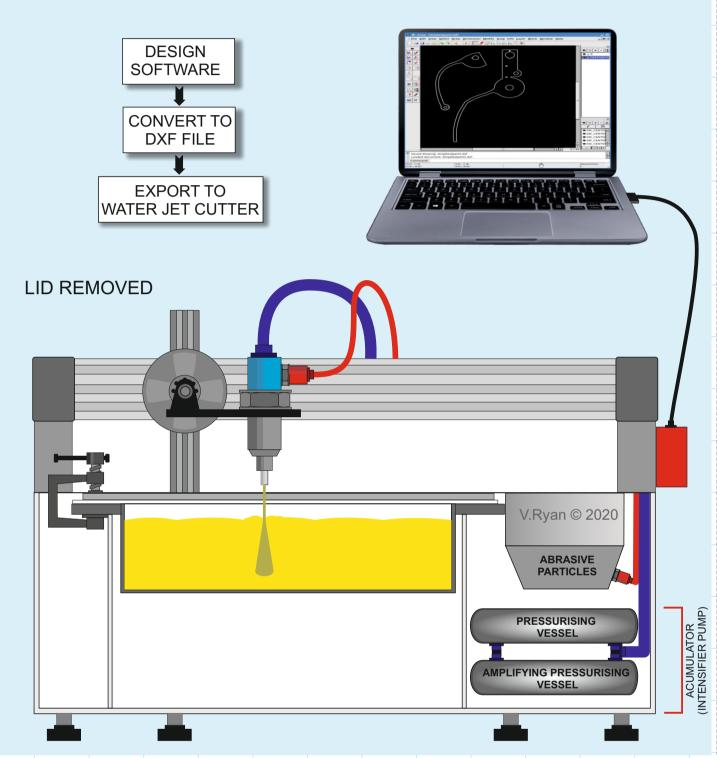
THE NOZZLE IS INTERCHANGEABLE AND FITS TO THE DYNAMIC HEAD. THIS MEANS THAT DIFFERENT WIDTHS OF **CUT CAN BE ACHIEVED. FINE CUTS AS** NARROW AS 0.5mm CAN BE ACHIEVED. THE WIDTH OF THE CUT IS REFERRED TO AS THE 'KERF'.
