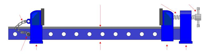
2. The box (below) is to be held together with sash clamps. On the diagram, draw a sash clamp in the correct position, across the box. Add explanatory notes.
