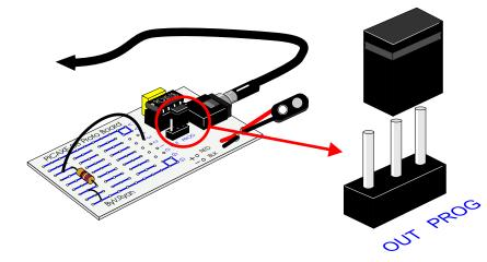
1. What is the function of the jumper switch, in a PICAXE 08 Starter board circuit?
