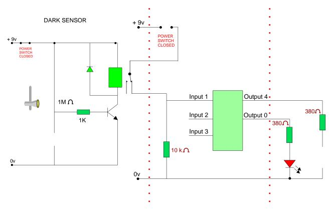
2. Explain / describe how this circuit works. The circuit has been designed to detect light / dark. It can operate as a light sensing or dark sensing device.
