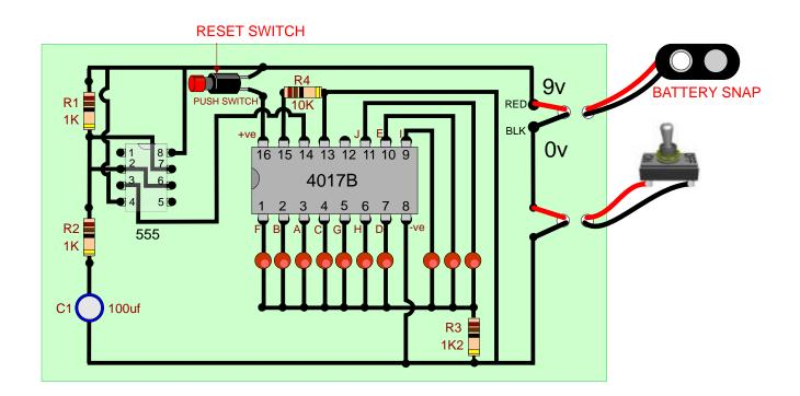
6. Below is a 3D view of the decade counter circuit. Label the components.
