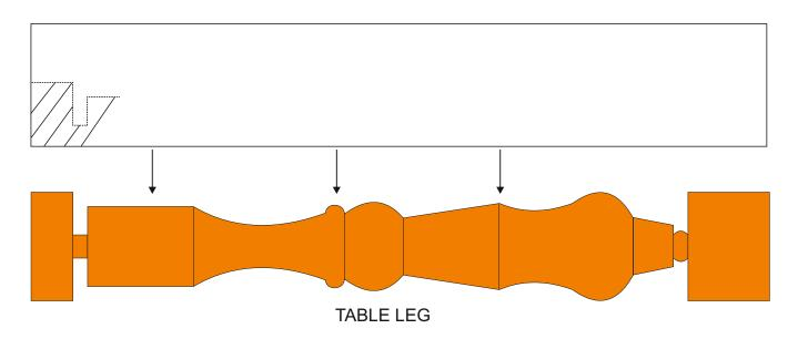
3. A card template is drawn below. Draw the shape of the completed piece of turned work. The first part of the finished product has been drawn for you.
