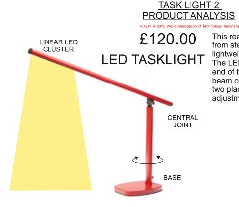
This reading light has a base manufactured from steel and 'arms' manufactured from lightweight round section aluminium tube. The LED cluster is arranged in a line, at the end of the upper arm, providing a wide beam of focussed light. It is adjustable in two places - rotation at the base and angle adjustment about the central joint.
