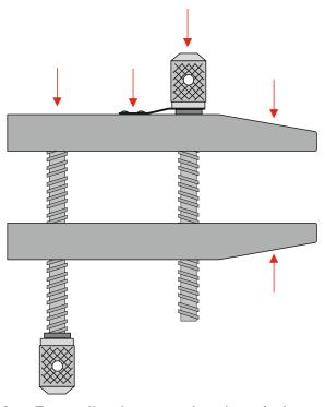
**2.** Complete the diagram of the toolmakers' clamp, by adding the labels indicated by the arrows. **5** *marks*
