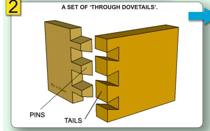
WHAT ARE THE BENEFITS OF USING **DOVETAIL JOINTS?** NAME TWO PRACTICAL APPLICATIONS OF THIS TYPE OF JOINT.
