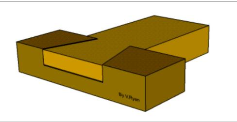
TEE HALVING AND HALF LAP JOINTS CAN BE USED WHEN GREAT STRENGTH IS NOT REQUIRED. SKETCH A TEE HALVING IN THE SPACE BELOW.
