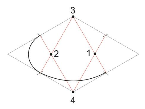
2. Draw isometric circles in the squares, using the compass technique. Do not erase any isometric guidelines you draw, to help you complete the question. 8 marks
