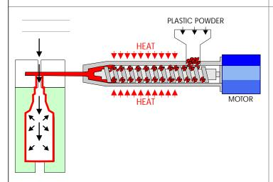
4. \_\_\_\_\_ air is 'blown' into the mould. This forces the liquid plastic against the sides of the \_\_\_\_\_. In this example it forms the shape of a plastic
