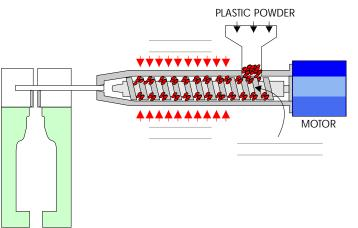
2. The \_\_\_\_\_ is turned on. This warms up and melts the granular plastic. A \_\_\_\_\_ turns a screw thread which pushes the granules along the heater section causing it to change to a
