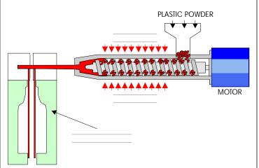
3. The liquid plastic is forced into a mould by
