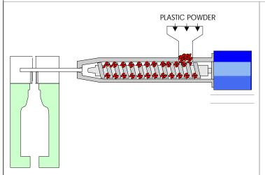
1. \_\_\_\_\_ of plastic powder (polystyrene, nylon, \_\_\_\_ and polythene) are poured or fed into a hopper which stores it until it is needed.
