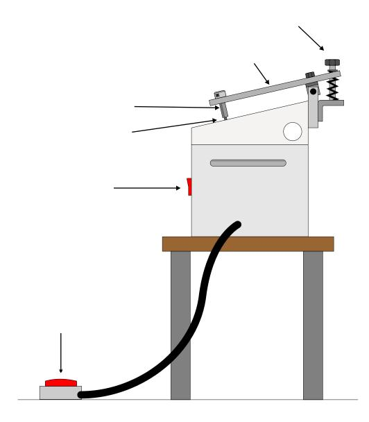
3. Why does a profile cutter have two switches? Remember, both switches must be pressed simultaneously in order for the machine to work.
