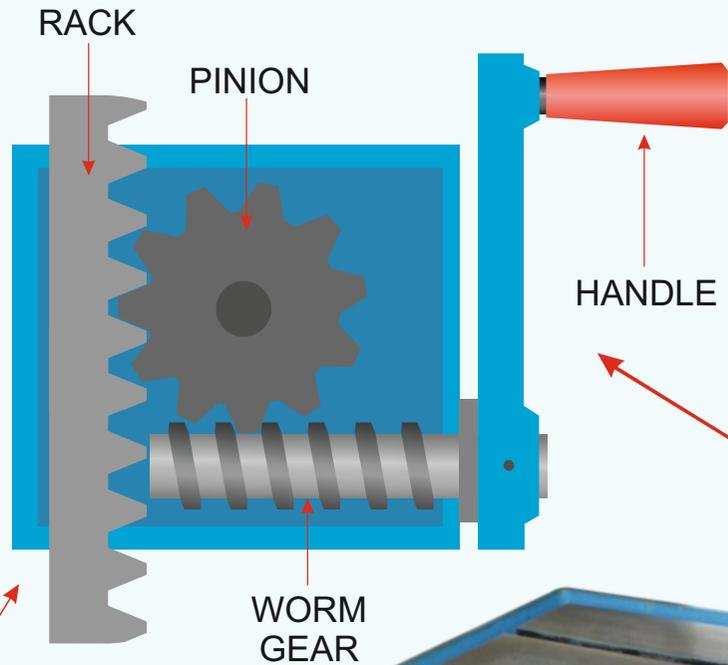
Rotating the handle, rotates the worm gear. The worm gear meshes with the pinion gear, which rotates. The pinion gear meshes with the rack, moving the machine table either up or down.
