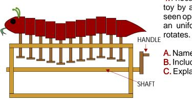
**4.** A local company has asked you to complete a mechanical toy by adding suitable cams. The partially made model is seen opposite. The flat followers rise and fall smoothly and at an uniform speed as the handle is turned and the shaft rotates.
