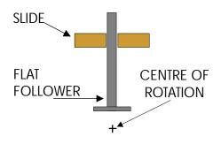
1. Complete the diagram shown opposite by adding a cam that has an eccentric profile.
