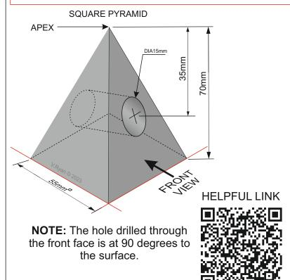
DRAW FRONT, SIDE AND **SECTIONAL PLAN ELEVATION OF** THE SQUARE PYRAMID SHOWN **ABOVE**
