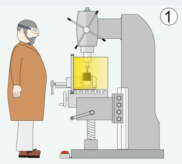
This is a Vertical Milling Machine. Identify all aspects that suggest that this machine is being used safely.
