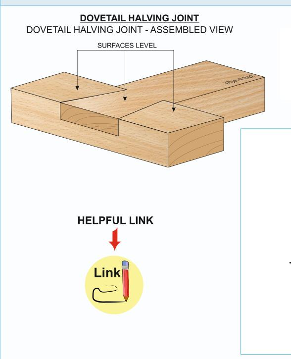
Detailed drawings of a common woodworking joint called a dovetail halving joint, are seen opposite.
