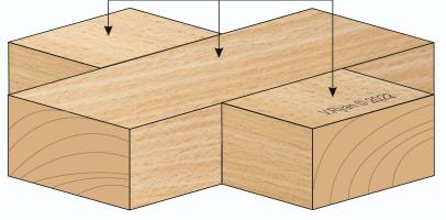
Detailed drawings of a common woodworking joint called a cross halving joint, are seen opposite.
