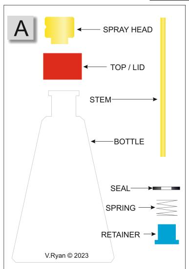
A disassembled perfume dispenser is shown opposite (Dia A). An assembled version is Dia B. You are to produce a, colour rendered, exploded drawing of the Dispenser, in the space below.
