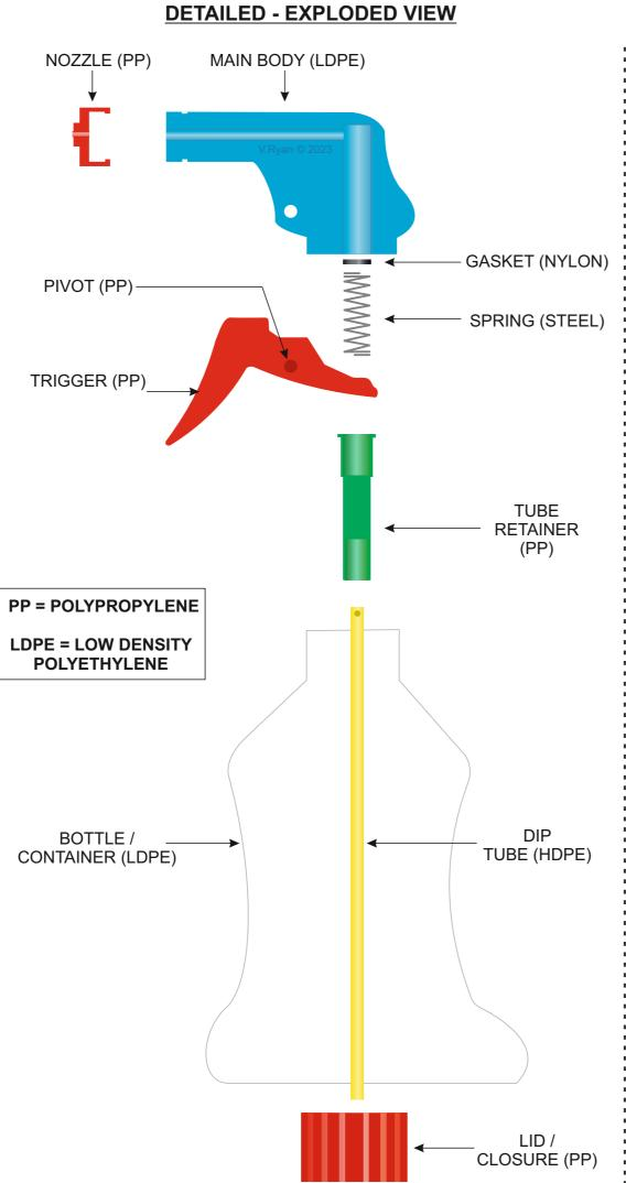
In the space below, draw an exploded view of the trigger action spray bottle. You can choose to draw a 'detailed exploded view OR an outline exploded view. Add labels identifying each part. (Please note - more marks will be awarded for the detailed view).
