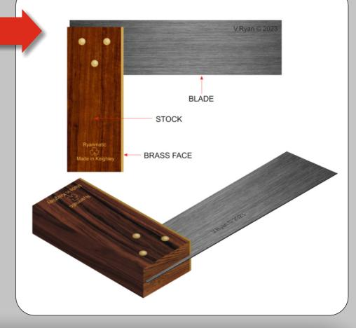
DESCRIBE HOW THE WOODWORKER'S TRY SQUARE IS USED TO MARK OUT MATERIAL
