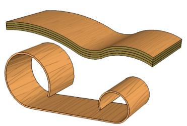
A flexible form of plywood. Can be formed into various 'curved shapes.
