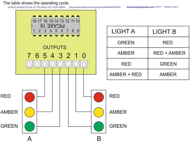
Outputs 0 to 5 are used to control the sequence of lights
