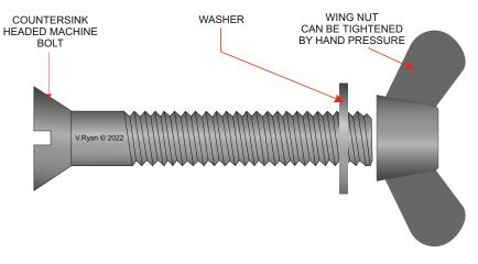
1. The bolt seen opposite is a Countersunk Head Machine Bolt. A wing nut is used in place of a typical nut. Give one advantage and disadvantage of using a wing nut.
